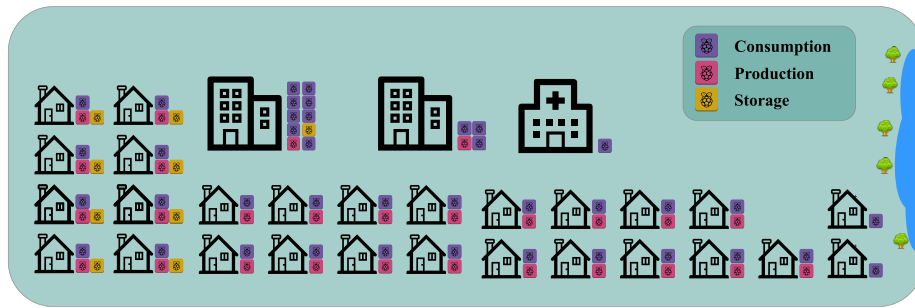
Fig. 1. Setup of the Walenstadt microgrid. The district consists of 37 participants with varying configurations. Two apartment buildings, eight prosumers with local storage, seventeen prosumers, two consumer households, as well as an elderly home as a large consumer.
